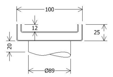
Our standard Tile Insert includes sizes 800mm, 900mm, 1000mm, 1100mm, and 1200mm with a fully welded 89mm spigot to centre.
